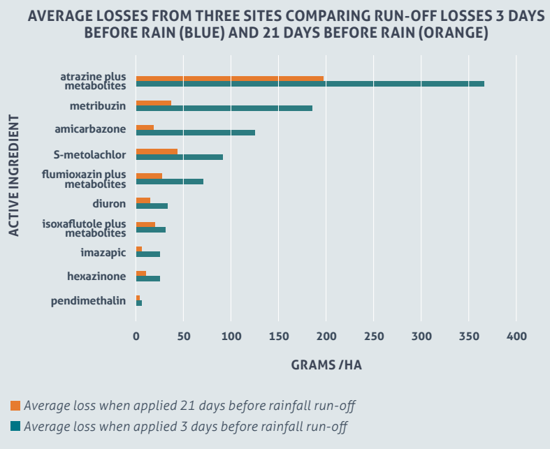
Figure 4: Effect of timing of first run-off on losses (Billing, B 2020). Extending the time from application to first run-off greatly reduced losses in surface run-off.
