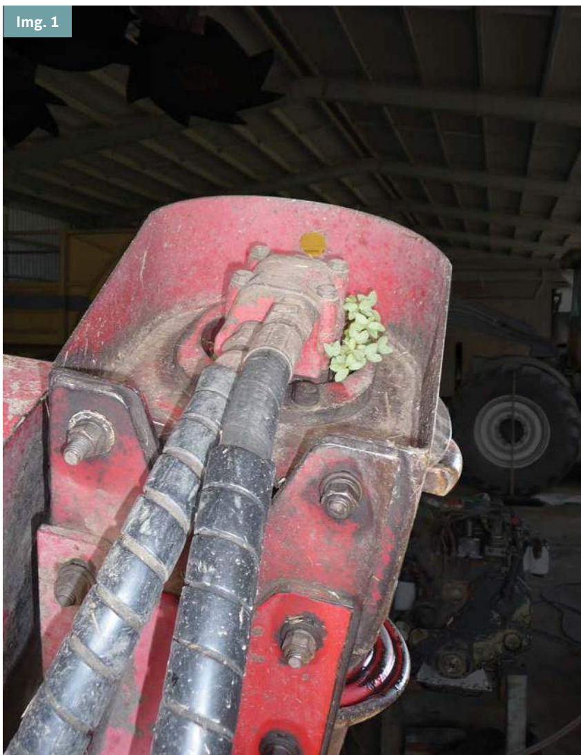
Image 1: Pink convolvulus seeds hidden on top of harvester spirals, after the machine was cleaned down.
