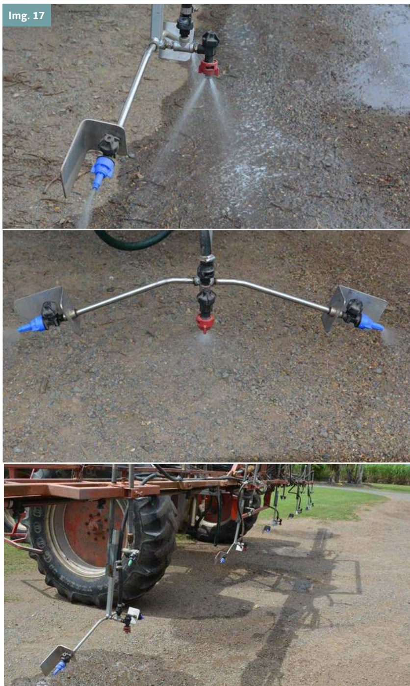
Image 17: Dropper and side arms custom-designed to replace Irvin trailing legs. Ray Abela, Eton
