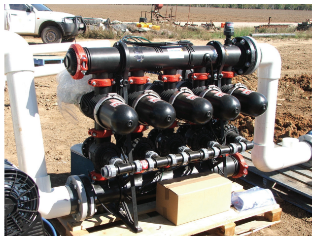
Above: Disc filters for a drip irrigation system. Photo courtesy of Steve Attard.
