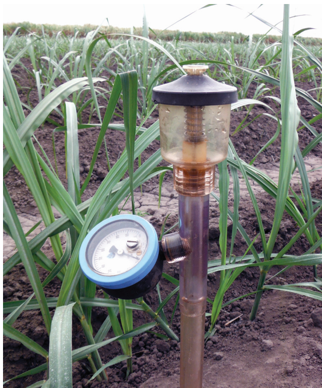
Above: Tensiometer installed in a field.
