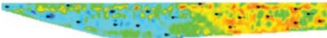
Figure 10: Use of EC mapping to determine appropriate sampling positions in a field
